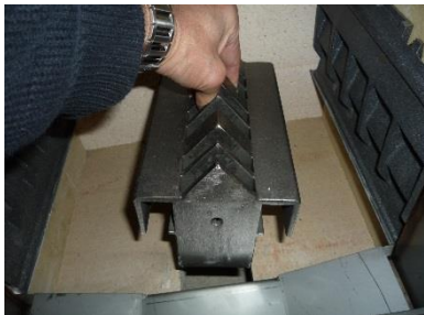
Injector block (Openings on the front/doorside)
